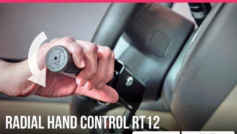
By pushing the grip downwards you accelerate, while by pushing the lever towards the dashboard you brake. Available both with interface and motor system.
